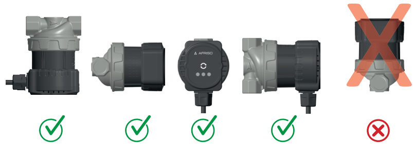
Fig. 2. Permissible mounting positions for the APW pump
