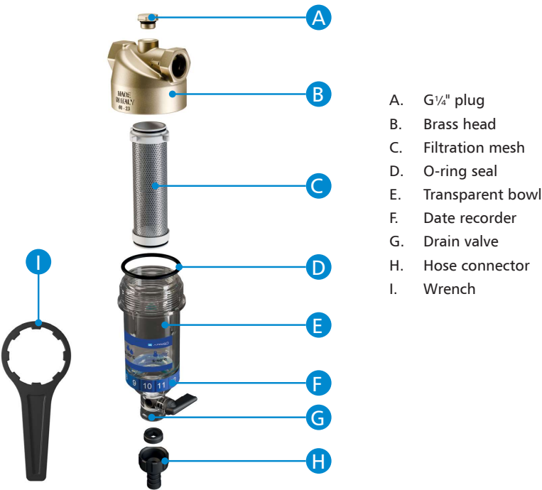
Fig. 2. Construction of the AWF water filter
