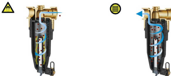
Figure 13. Stages of medium filtration in the ADS 181 separator
