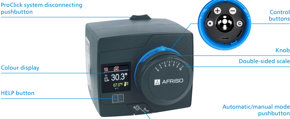
Fig 1. Construction of the ACT ProClick constant temperature controller
