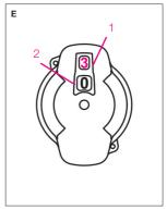
Use of the balancing valve: setting the flow rate (fig F-G)
