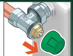
To pre-set the flow rate, place the specific shaped ring.
