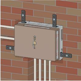
The protection cover protects the inner parts of the box during installation procedures.
