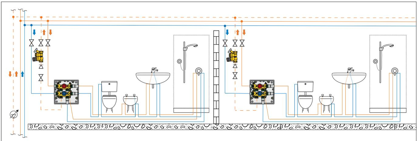
**Centralized system: hotel / hospital with a high level of automation (production with storage and peripheral hot/cold recirculation circuit)**
