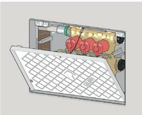
Secure the inspection port frame to the box, adjusting its depth with the special adjustment screws until it is flush with the wall.
