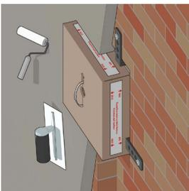
The cover provides a reference for the area to which the surface finish of the wall needs to be applied in order to achieve perfect alignment of the cover plate.
