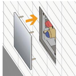
Fasten the aesthetic cover plate to the cylindrical guides.
