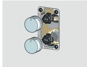
Secure the knobs using the relevant fixing screws and push on the chrome plated covers until they click into place.
