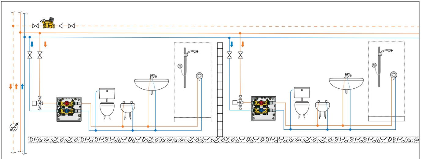
**Pass-through loop distribution and bathroom recirculation**
