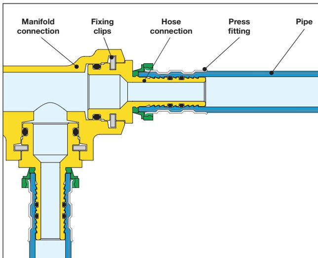
Insert the pipe, including the fitting, into the slot on the manifold.
