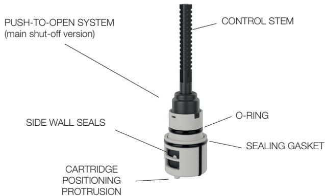
There are cartridges of two types and sizes, one used in manifolds with individual shut-off valves and one designed for versions with main shut-off valves. The version used for in-wall main shut-off valves features a stem with a push-to-open system. It helps to achieve the concealed effect for the knobs used to move the cartridge.
