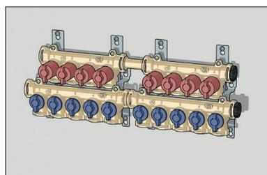
Fit the lower manifold on the wall.
