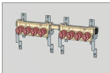
Fit the upper manifold and position the brackets for the lower manifold.
