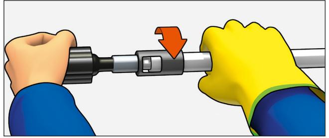
After calibrating the pipe using the relevant calibrator, push the pipe onto the fitting, making sure it reaches the end point. You should look through the windows to make sure the pipe is in the correct position.
