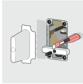
Remove the mask protecting the shut-off valves and use the built-in template to cut the stems, in order to achieve correct alignment of the knobs.
