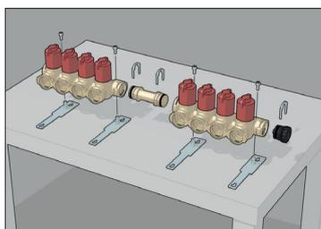
Assemble the upper manifold in the desired configuration.
