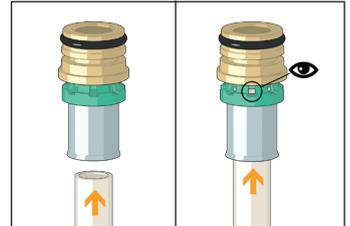
Clamp the pipe using the relevant clamp, until a click sounds automatically.
