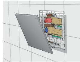
Fix the cover plate to the support plate.
