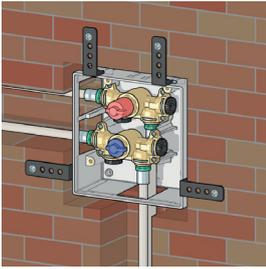
The wall-mounting box is installed in the same way as for the in-wall version.
