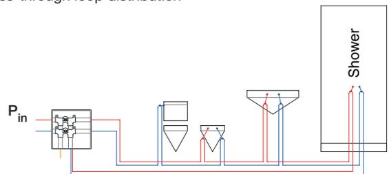
For a detailed calculation of the pressure drops within the loop circuit, please refer to the H. Cross method.
