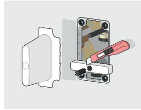
Remove the mask protecting the shut-off valves and use the built-in template to cut the stems, in order to achieve correct alignment of the knobs.
