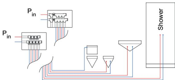
Manifold with individual shut-off valves
