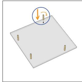
Screw the pins to the rear of the plate.
