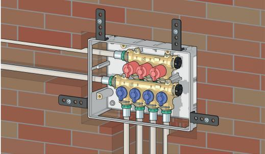
The protection cover protects the inner parts of the box during installation procedures. It also provides a reference for the area to which the superficial finish of the wall needs to be applied in order to achieve perfect alignment of the inspection port or cover plate.
