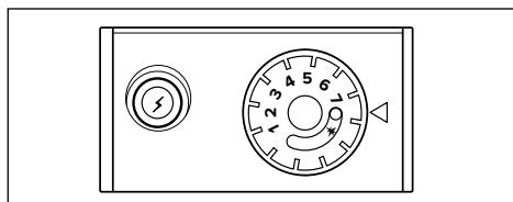
Press knob B fully in and hold it there; now press the piezoelectric igniter C. Check for a flame though hole A. Once the flame is on, continue holding knob B pressed in for a further 20 seconds or so. If the pilot flame does not stay on, repeat the above procedure.
