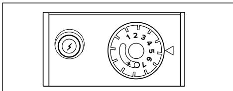
To reduce gas consumption and run the appliance more efficiently, it is best to leave the knob at setting 5 (around 60°C).
